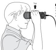
NOTE This product contains a built-in orientation sensor to assure proper usage. If the T10 is in an improper position for usage, (upside down) the unit will beep repeatedly until the correct orientation is restored.
