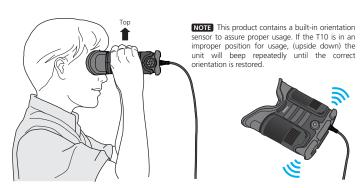
With the visor in position, look straight into the unit so that the left eye is centered in the mirror. (During the enrollment process the eyes should be open as wide as possible until the capture process is completed)
